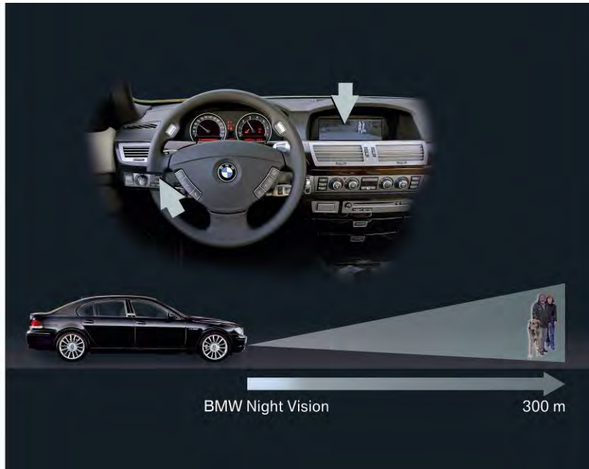
Figure 5.2 Night vision system of BMW (BMW press archive). Range of the system, monitor placement and activation command (arrow to the left of the steering wheel) are shown.
