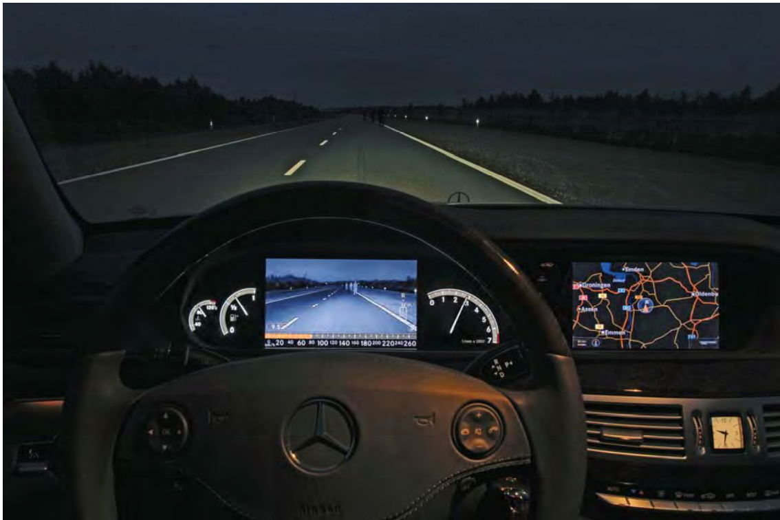
Figure 5.4 Night vision system in Mercedes cars showing the screen with image produced by the night vision system in the centre line of the sight (near tachometer) as seen by the driver through the steering wheel.
