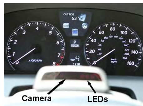
Figure 5.1b Device with camera and LEDs in the Lexus LS 600h to monitor the drive (figure adapted from www.autospies.com ).
