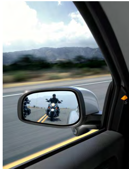
Figure 5.13 Volvo BLIS system in a situation where the driver would receive a warning that other vehicles are on the side of the car. Warning light is visible in orange. (Volvo Car Corporation Newsroom.)
