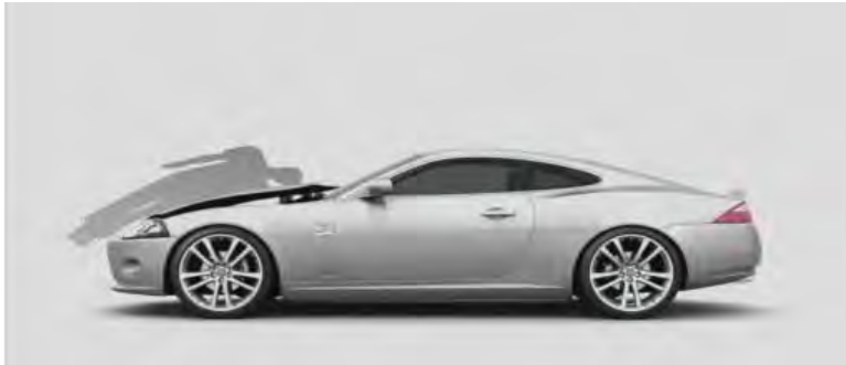
Figure 5.18 Jaguar deployable bonnet system. Bonnet is seen lifted in case of impact with pedestrian (figure from Jaguar press release).
