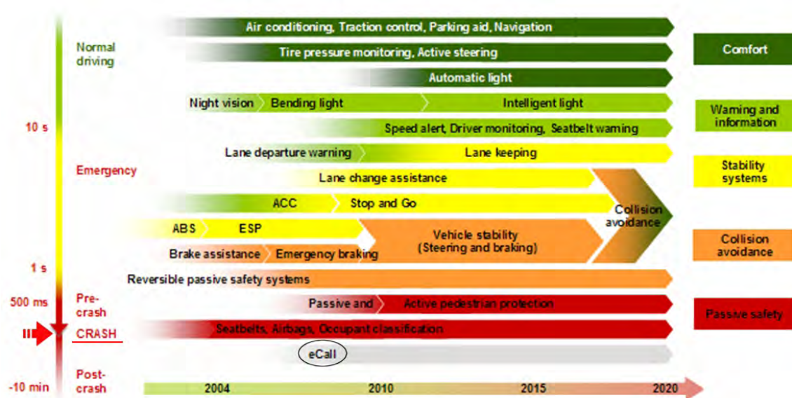
Figure 4.7 ITS roadmap adapted from Abele et al. (2005). Timeline raises on the x-axis, while driving situation is colour coded on the vertical line, with red colour signifying crash situations, yellow meaning emergency situations, and green colour normal driving situations. The colour coding denotation is reflected in the system function.
