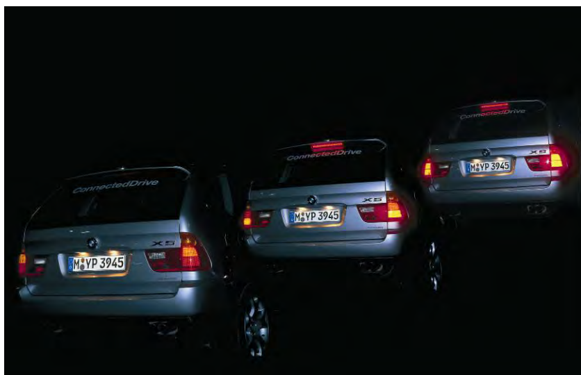
Figure 5.5 Brake force display (BMW press archive). Left car: without applying the brakes (only lights on), middle car: applying the brakes normally, right car: applying the brakes hard. The intensity of the brake lights is higher in the right car, signaling stronger deceleration.
