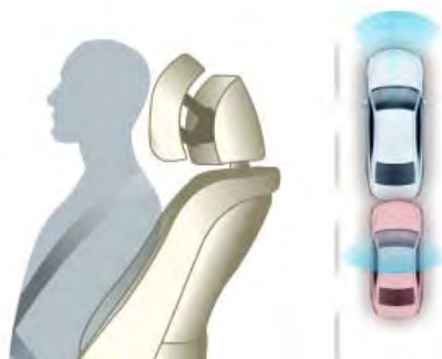
Figure 5.17 System activation before imminent rear-end crash. The head restraint moves toward the driver’s head to reduce the risk of whiplash injuries. Figures adapted from www.lexus-europe.com .
