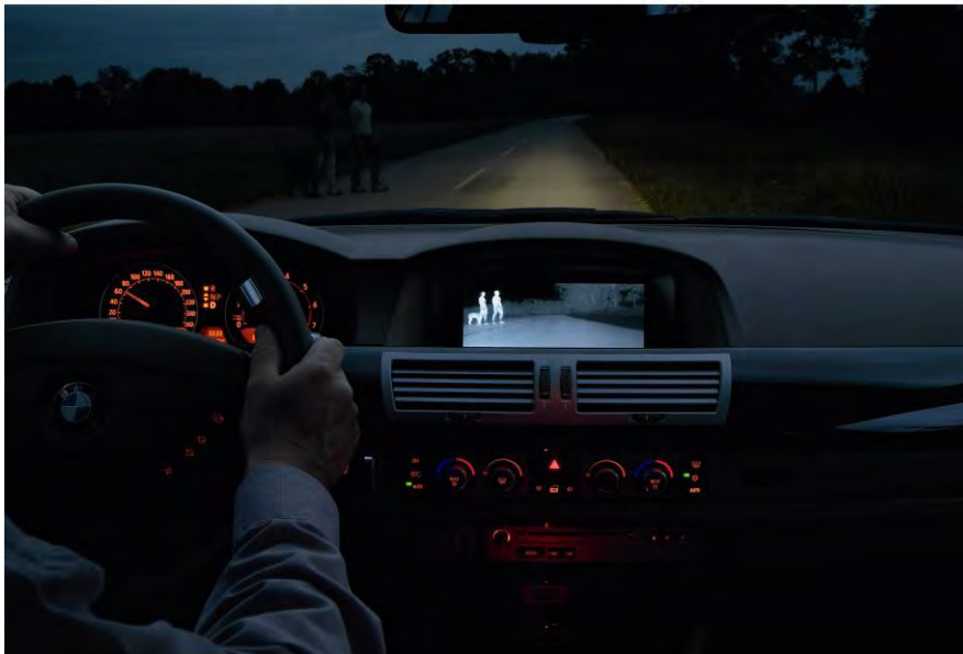
Figure 5.3 Detail of the night vision display (BMW press archive). The monitor (in greyscale) shows the pedestrians with a dog that would otherwise be more difficult to detect by the driver when only looking through the windscreen.
